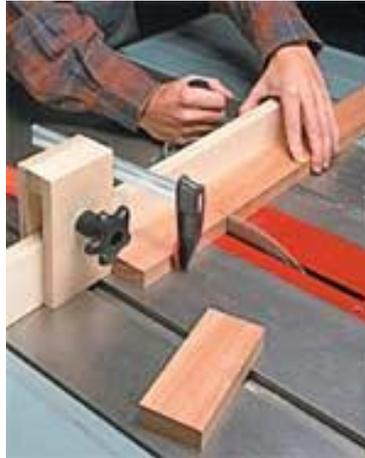
Stop blocks are an indispensable accessory when cutting pieces to length on the table saw or miter saw. And they don't get much simpler or quicker to make than this one.
