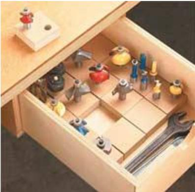
As my router bit collection grew, I needed an easy way to organize the bits and protect the carbide cutting edges. So I came up with a modular organizing system, see photo.
