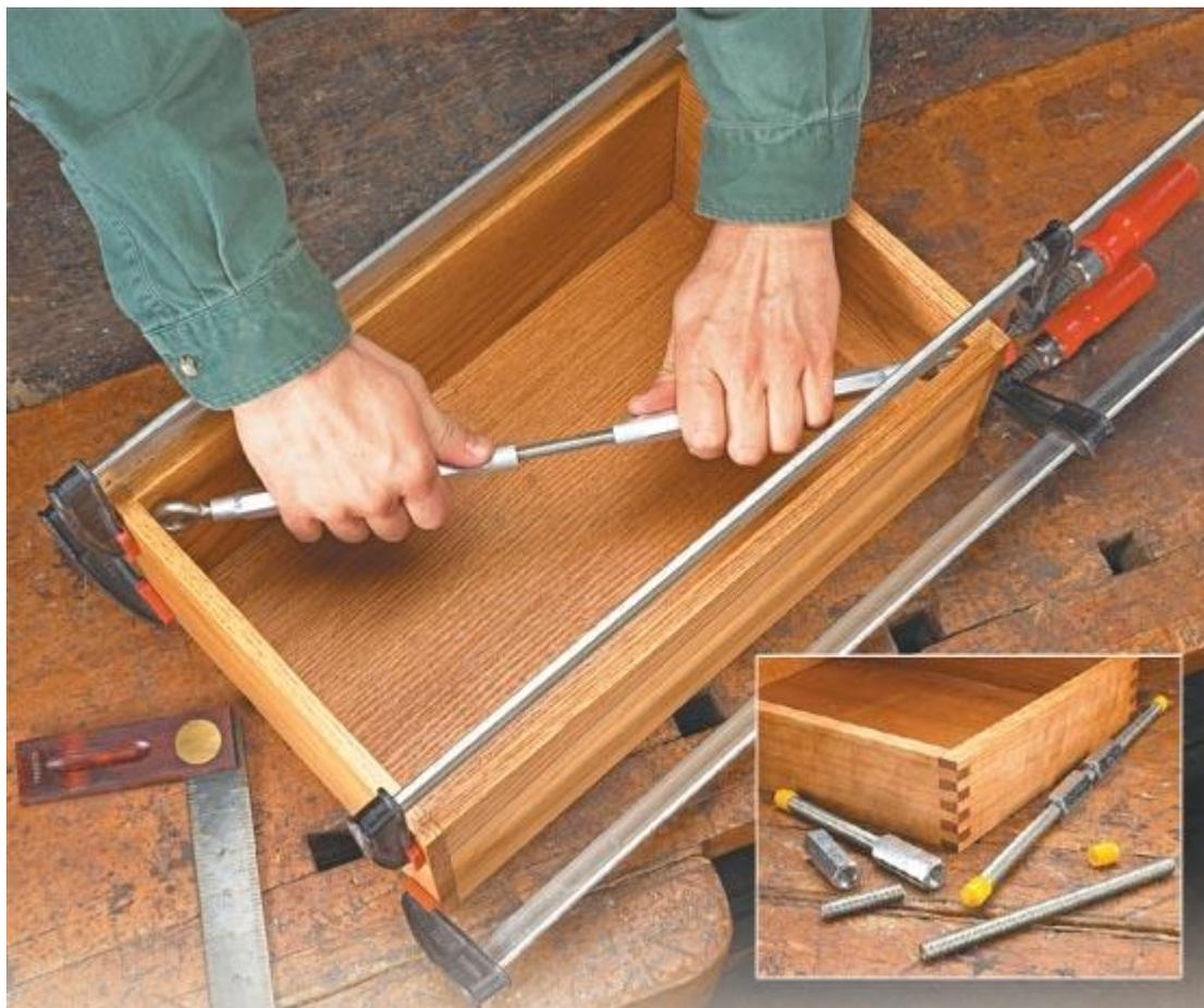
The concept is pretty simple. The squaring rods are used to apply pressure across the short diagonal of the drawer to push it into square. For large drawers I have a squaring rod consisting of a section of threaded rod, two turnbuckles and a couple of eyebolts. As you can see, the eyebolts wedge into the corners of the drawer to force it into square.
